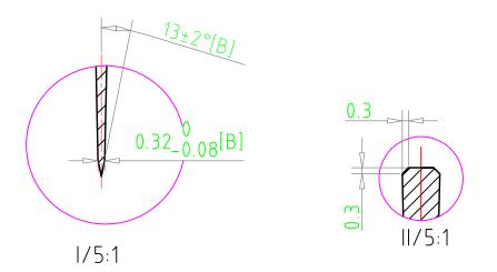
Tolerance unless otherwise specified 0-3mm ±0.5 >3-30mm ±1 >30-120mm ±1.5 >120mm ±3 The line of the logo (etching technology) must be uniform.
