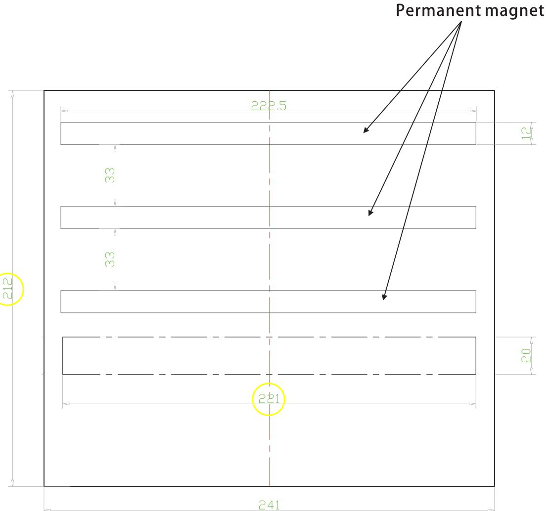
Surface treatment: three layers of varnish treatment Specification:
