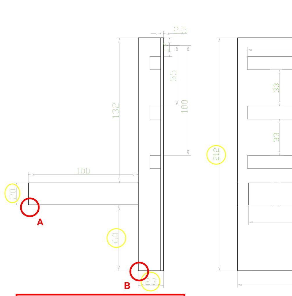
The edges A and B must be parallel.
