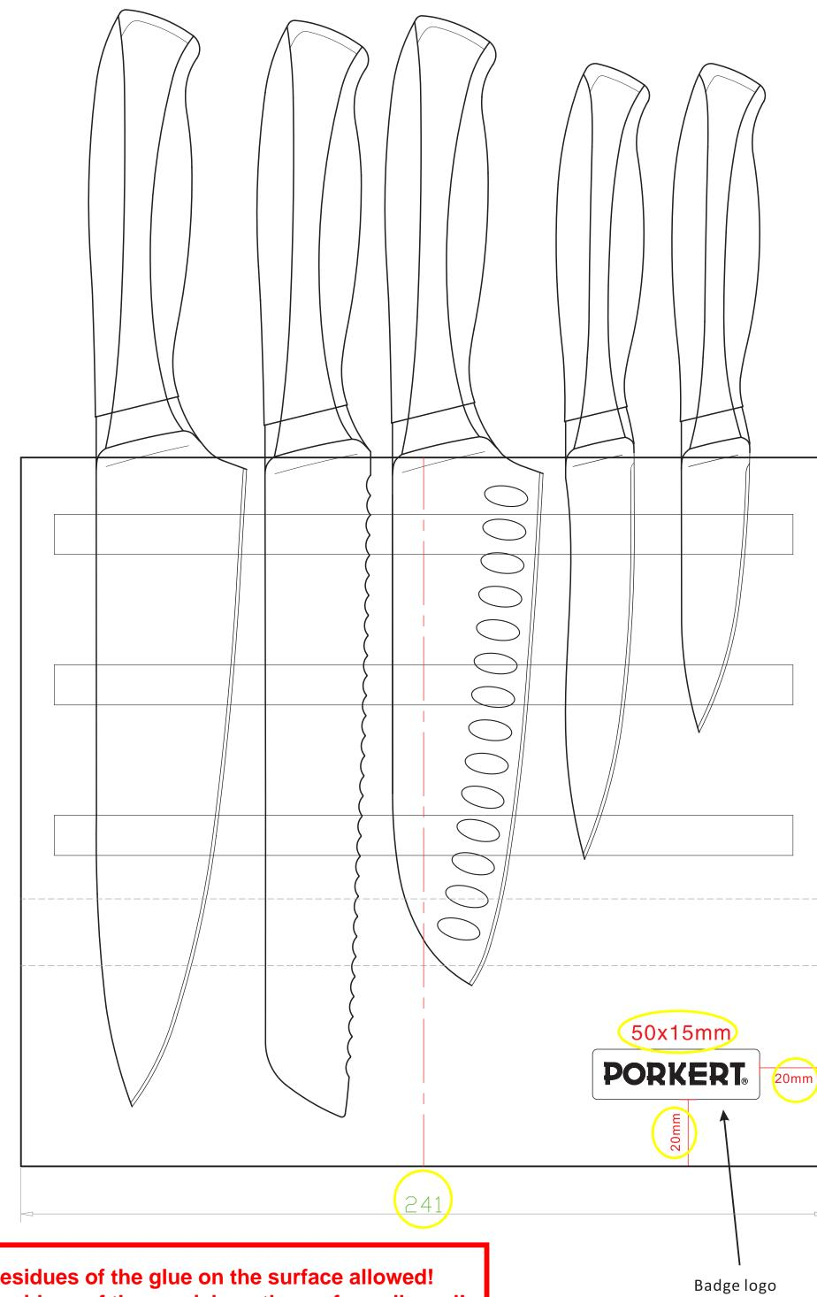
No visible residues of the glue on the surface allowed!
